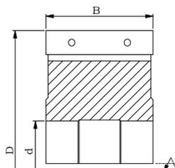
$D_{max} = 400 \text{ mm}, B_{max} = 120 \text{ mm}$
